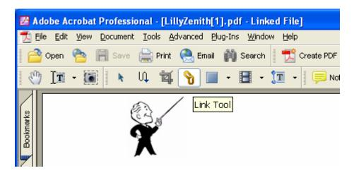
Any text, image, or area of the PDF document may be a hyperlink using this tool. Select the tool, then click and drag to create a box around the desired area for the hyperlink. The *"Create Link"* dialog is displayed:
